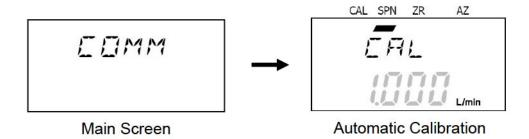
For the MP-W5P model, if no key has been operated for 30 seconds or more, the pump enters a sleep mode that prevents communication. If that occurs, press any key except the [START/STOP] key on the MP-W5P unit before pressing the [ENTER] key on the FC-M1 unit.
