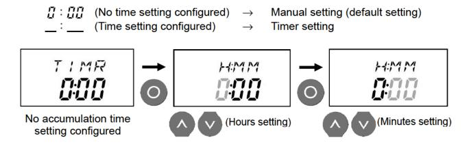
Press the [ENTER] key, which causes the hours display (hours) to flash. Then use the [UP] or [DOWN] key to set the time (hours). Once again, press the [ENTER] key, which causes the minutes display (minutes) to flash. Then use the [UP] or [DOWN] key to change the setting for minutes. Press the [ENTER] key to confirm the setting. (To return to the previous screen without changing the setting, press the [MODE/ESC] key.)
