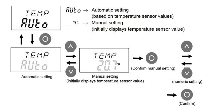
Press the [ENTER] key, which causes the display to flash, then use the [UP] or [DOWN] key to select auto or manual mode. In the manual mode, press the [ENTER] key again and then the [UP] or [DOWN] key to change the temperature value. Press the [ENTER] key to confirm the setting. (To return to the previous screen without changing the setting, press the [MODE/ESC] key.)
