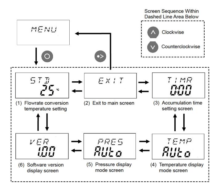
Press the [MODE/ESC] key to return to the [MENU] screen from any sub-screen in the dashed line area above.
