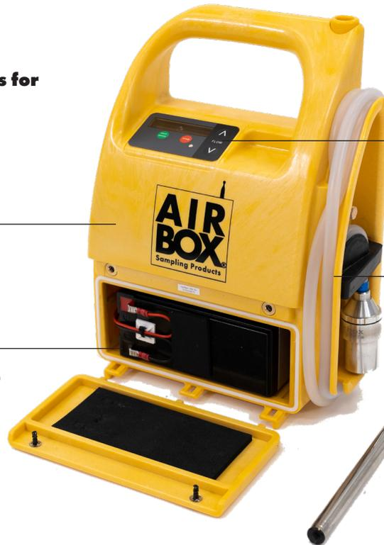
**Easy to use control panel with highly visible OLED display**
