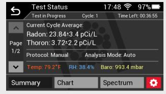
Alpha spectrometry measurements are used to determine radon and thoron concentrations:
