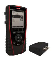
MP 210 P: MP 210 + MPR 500 pressure module (±500 Pa pressure module)
