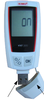
Data collector – PC connection
