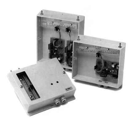
The **ECM** electric contact pressure controllers are the result of a long experience in the research and manufacture of measuring and control instruments. They are designed to combine the inherent reliability and accuracy of the liquid column manometer with electronic switching.
