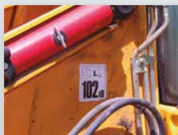
Statement of noise produced by machines and indication of sound power level
