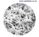
nfo@sedulitas.co.za www.sedulitas.co.za www.sedulitas.co.za Polyvinyl Chloride (PVC) Membrane Filters are excellent membrane filters for sampling airborne metals, silica, and dust. Comprised of inherently low ash pure homopolymer PVC, these filters are particularly well suited to provided interference-free silica determinations. Low moisture pick-up and low tare weight assure gravimetric stability.
