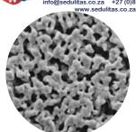
Silver Metal Filter Membranes are pure metallic silver (99.97% pure silver) and are available with particle retention ratings of 0.45 or 0.8 microns. Silver metal membranes are used in a variety of filtration applications, and their ability to withstand extreme chemical and thermal stress makes them ideal for applications involving aggressive fluids and/or high temperatures.
