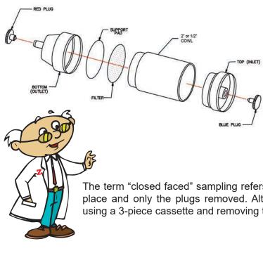
3-piece asbestos style cassettes feature a 2" (50mm) or 1/2" long cowl and can be used for both "open face" and "closed face" sampling. These housings are available with a static conductive cowl or in a clear styrene material.
