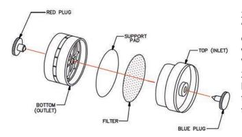
2-piece cassettes are advantageous when only "closed faced" sampling is required. This is because during sampling, contaminants will cling to the walls of the cassette from electrostatic forces. With approximately 35% less surface area in a 2-piece cassette vs. a 3-piece cassette, there is less surface area for contaminants to cling to and thus more contaminant where it should be — on the filter membrane.
