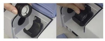
A dust sample is first collected using traditional samplers. The sampling cassette is removed and placed in a portable Fourier-transform infrared (FTIR) instrument in the field. The FTIR instrument examines the dust sample and offers a complete analysis in one to two minutes. Source: Emanuele Cauda, PhD; Lauren Chubb, DrPH; and Valerie Coughanour, MA, MFA. https://blogs.cdc.gov/niosh-science-blog/2018/02/21/engineers-week-mining.
