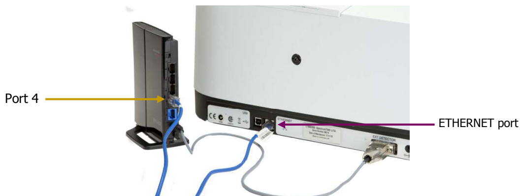
Figure 17 Ethernet cable connected to Port 4 on the wireless router and the Spectrum Two
