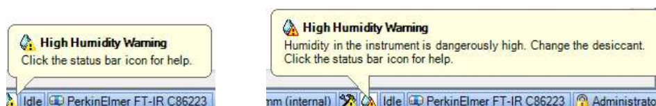
Figure 72 Humidity sensor High and Critical warning messages
