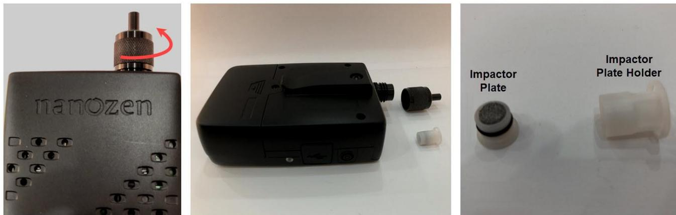
Figure 1 Impactor Assembly: Impactor Cap, Impactor Plate Holder and Impactor Plate.
