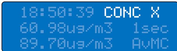
Figure 30 Concentration alarm (CONC) with audible and visual alarms disabled as displayed on the LCD
