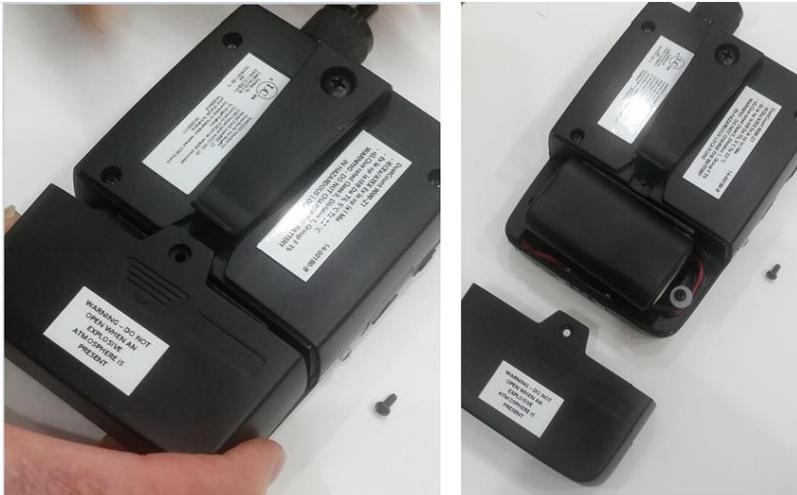
Figure 81 Sliding off Rear Battery Cover
