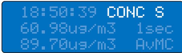
Figure 29 Concentration Alarm (CONC), with audible and visual alarms enabled as displayed on the LCD in Classic Mode
