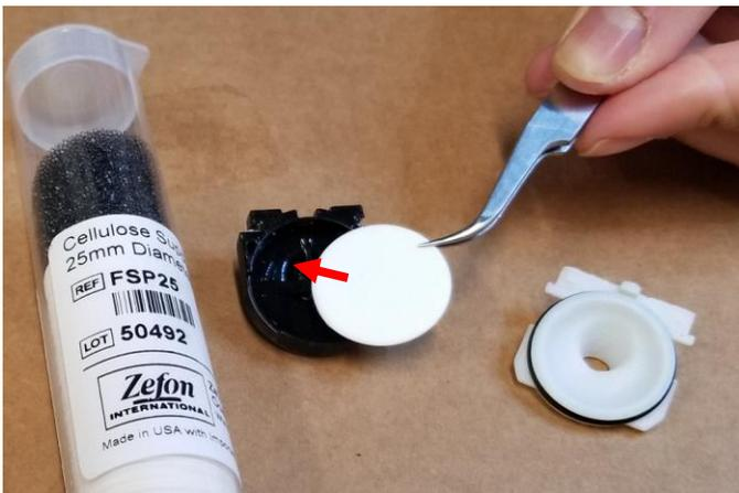
**Figure 14** Installing Fiber Support Backing with Tweezers
