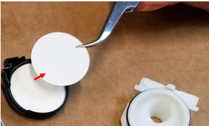
Figure 12 Filter Exposed for Removal. Slide Filter Out of Cavity with Tweezers
