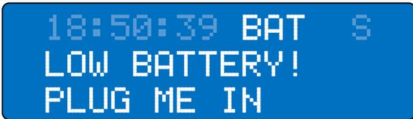
Figure 32 Shutdown (0 - 1%) Battery State-of-Charge as displayed on the LCD
