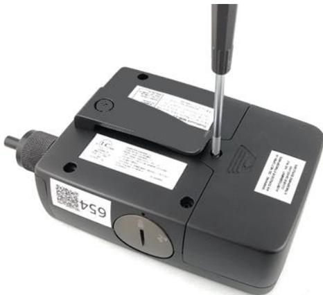
**Figure 80 Loosening and removing Screw for Rear Battery Cover**
