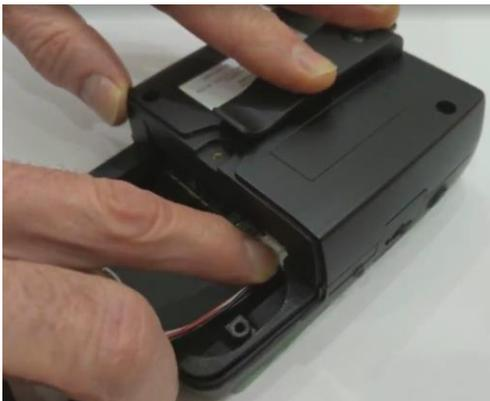
Figure 83 Press Down on Tab to Disconnect Battery
