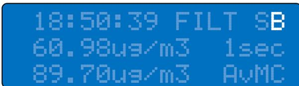
Figure 45 Bluetooth Connected displays B at the top right corner on the LCD
