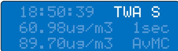
Figure 39 Time-Weighted Average Alarm (TWA) displayed on the LCD
