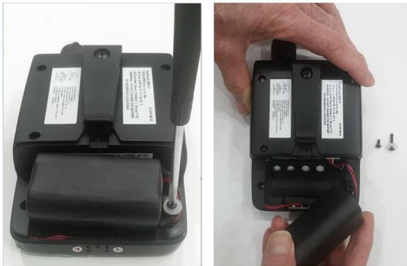
Figure 82 Removing Screw to Release Battery Cable Tie
