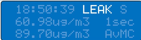
Figure 35 Leak detection alarm (LEAK) displayed on the LCD
