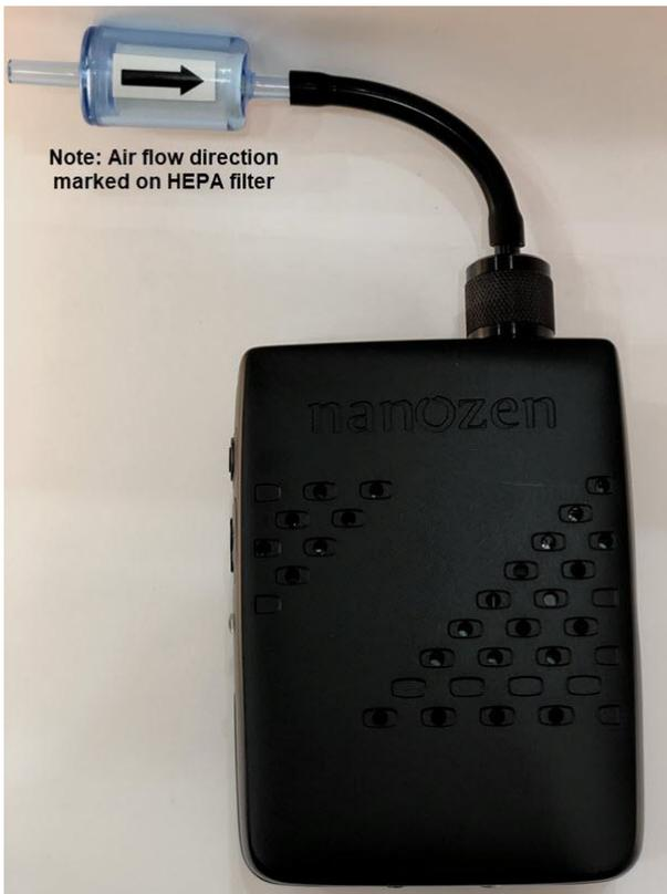
Figure 7 HEPA filter connected to the DustCount IS input
