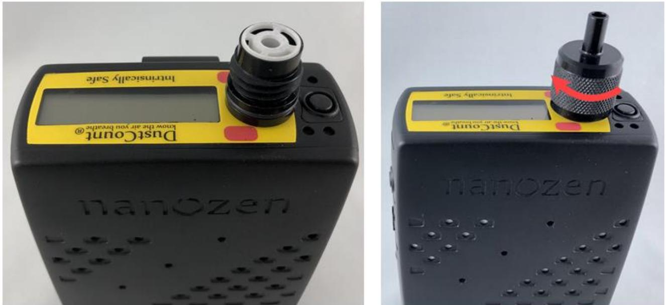
Figure 6 Insert Impactor Plate holder assembly into Impactor base and screw Impactor Cap onto the base.
