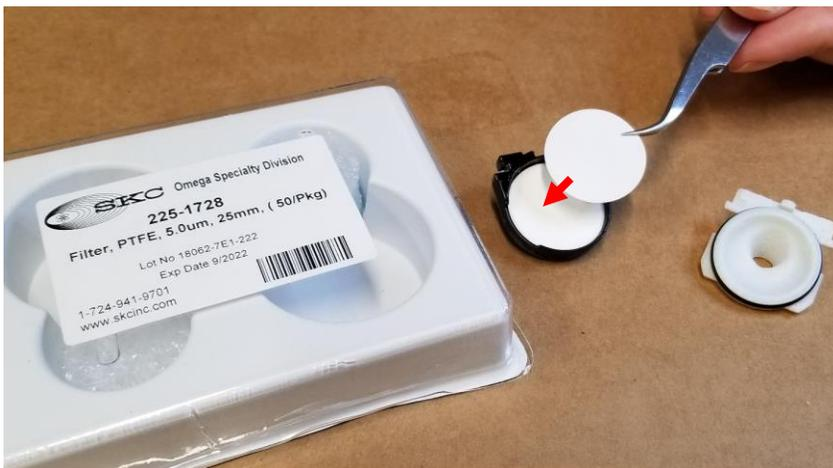
**Figure 15** Installing Filter with Tweezers on top of Backing
