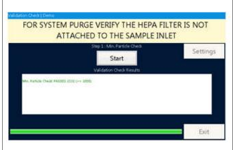
Remove the HEPA filter or the mask if attached, and tap the [Start] button to check that the particle concentration in the ambient air is sufficiently high enough to calculate the mask fit factor. Depending on the ambient particle concentration (i.e., outside of the mask), the environment may be inappropriate to perform a mask fit test. This process also confirms that the device is operating properly. When this measurement is complete, proceed to the Zero Check
