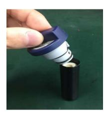
2) After the cartridge is separated, use the felt removal tool (a small wooden stick) to push the felt and mesh out of the cartridge cylinder (Figure 2).
